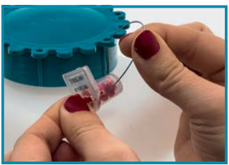
Insert the seal wire through the holes of both the cap and bottle itself. Then insert the wire into the hole of the seal as shown.
