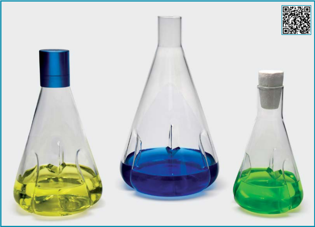
Featured with 4 integrated baffles for efficient mixing. Baffles create a turbulent flow, enlarge gas exchange surface and increase oxygen intake.
